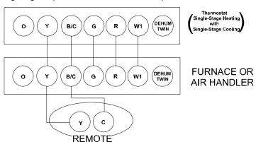
Single-Stage Thermostat with Two Low Voltage Wires to Remote
